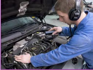
Designed to allow the user to listen to amplified sounds through a professional set of headphones during a road test.
