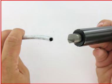
An essential tool for ensuring brake pipe are deburred effectively.
