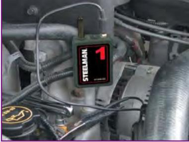
Quickly pinpoints source and location of noise during a road test, even on long vehicles (such as trucks, buses...).
