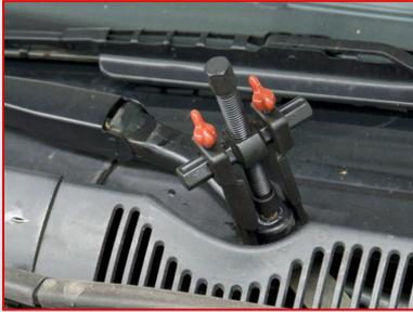
Contains many accessories (including a universal puller) that will assist with the removal of wiper arms that are:
