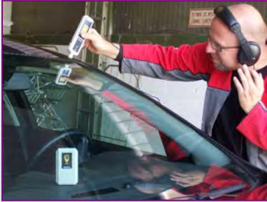
**Quickly find air and water leaks within the vehicle.**
