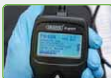
Displays Diagnostic Trouble Code (DTC) and definition.
