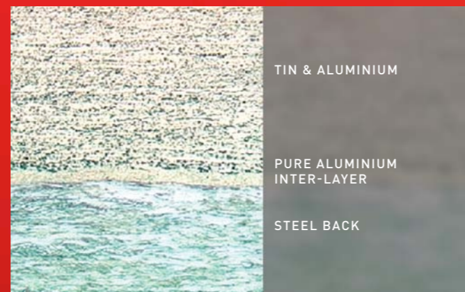
[FIG.32] CROSS-SECTIONAL CUT THROUGH A BEARING SHELL MADE OF A370®. THE PURE ALUMINIUM INTER-LAYER BONDS THE TIN-ALUMINIUM ONTO THE STEEL BACK.
