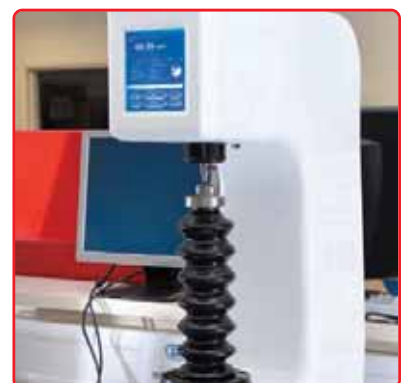
measuring hardness of the striking face
