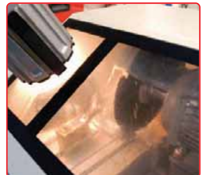
Hammer head is sliced to facilitate hardness testing of both the striking face and at 3mm depth
