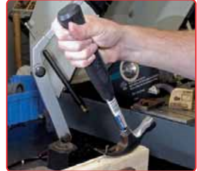
Nail extraction test for claw hammer
