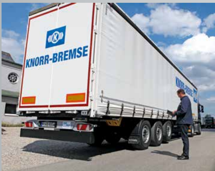
iTAP enables the driver to easily control trailer functions remotely.
